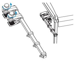
Step 3: Using the screws, tighten the bracket to clamp onto the awning arm. Tighten enough to ensure there is little to no movement of the clothesline bracket.
